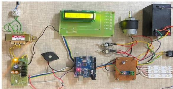
Fig No. 10 Working prototype model of Smart BMS
