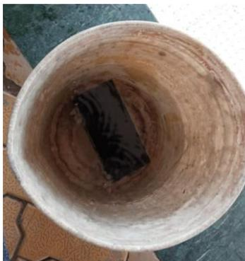
Fig 3.3: Water absorption test
