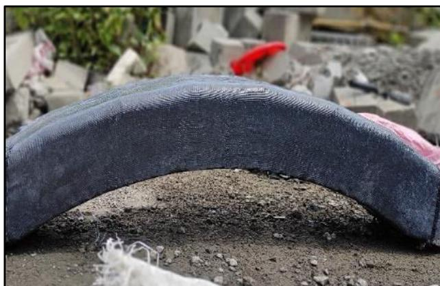
Figure 1b Wrapping of Specimen
