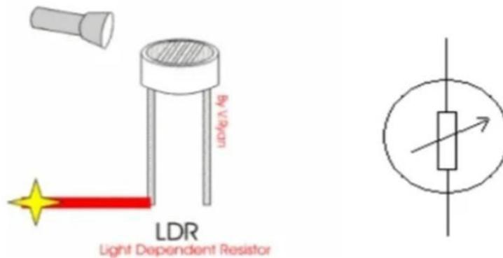
Fig. 3. Light Dependent Resistor
