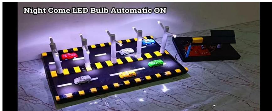
Fig. 11. Automatic Street Light Prototype
