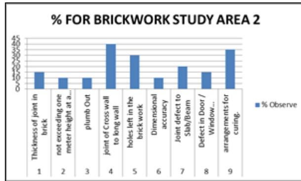
Fig 7 for Brickwork Defects Study Area 2
