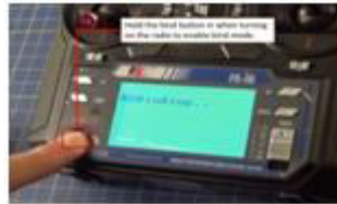
Fig.14 Bind and setup for Radio controller
