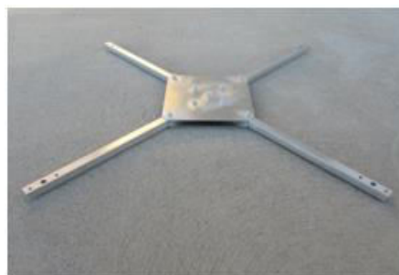
Fig.7. Quad-copter made with aluminum Frame
