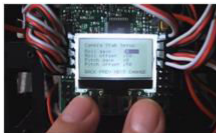
Fig.9. KK 2.0 flight controller setup
