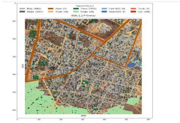
**Figure 2 :** Impervious Surface Extraction Results From Experiments.
