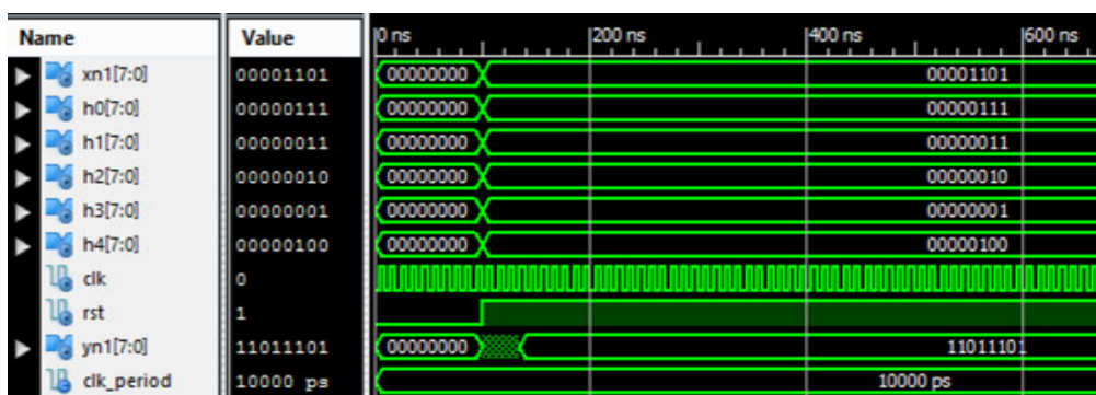
Fig. 5: Output Test Bench Waveform of Narrow Band Filter (Filter Coefficient N=5)
