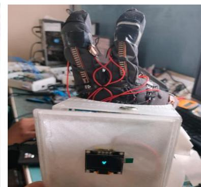
Fig.13 Letter 'V' on OLED display
