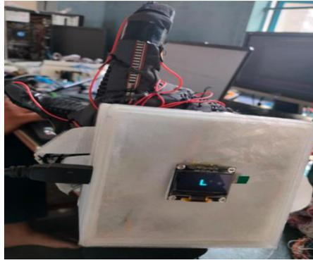
Fig.9 Letter 'L' on OLED display
