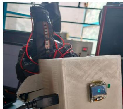
**Fig.6 Letter 'D' on OLED display**
