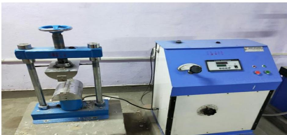
Fig.5 Split Tensile Strength Test Machine
