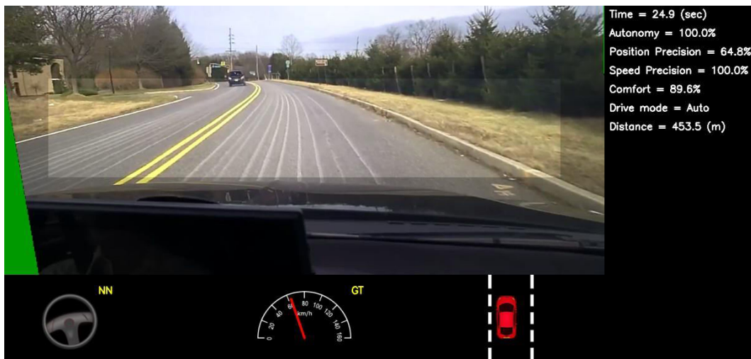
Figure 6: Screen shot of the simulator in interactive mode. See Section 7.1 for explanation of the performance metrics. The green area on the left is unknown because of the viewpoint transformation. The highlighted wide rectangle below the horizon is the area which is sent to the CNN.
