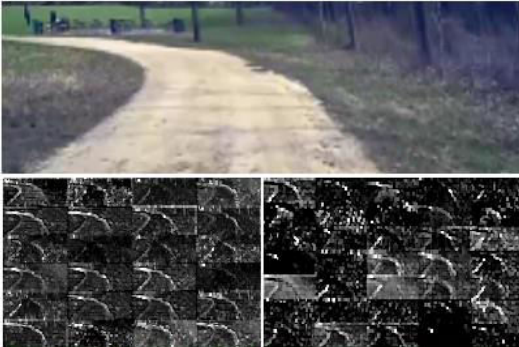
Figure 7: How the CNN “sees” an unpaved road. Top: subset of the camera image sent to the CNN.
