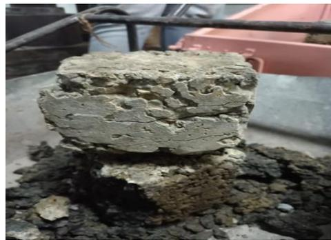
Fig.6 15% air content cube after compressive test
