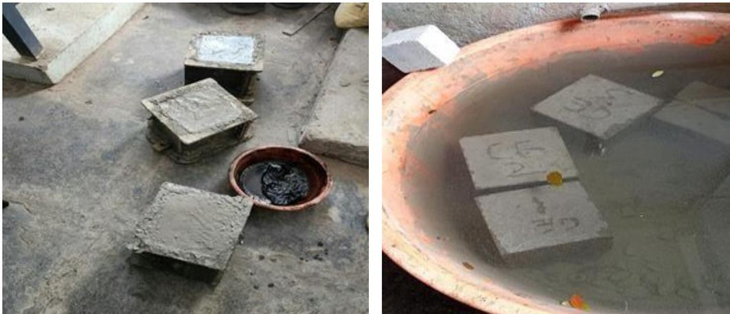
Fig.2 Concrete fill in mould and put in the water for curing
