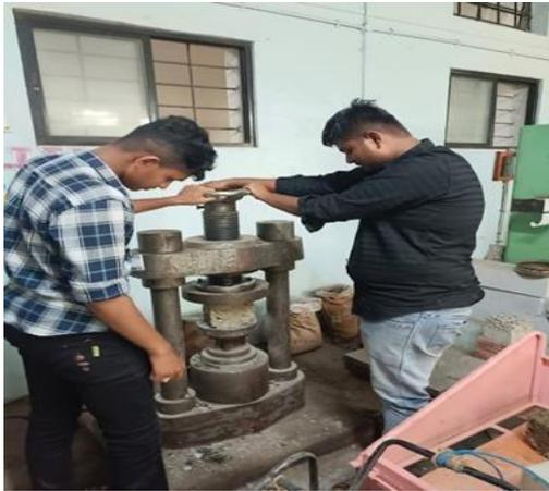
Fig. 4 Place the concrete block between two plates
