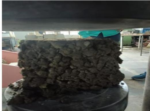
Fig.7. 20% air content cube after compressive test
