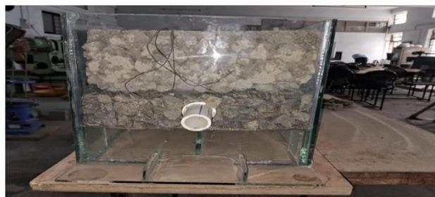
Fig. 2 Model of pervious concrete
