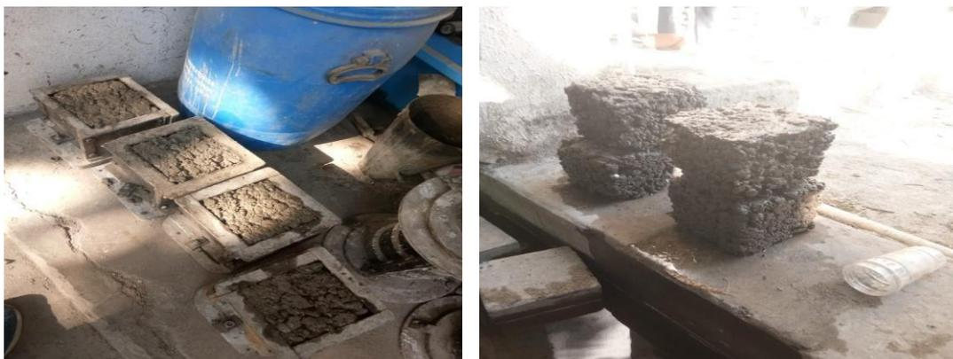
Fig. 1 Permeable concrete in fresh and hard condition
