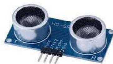
Figure 2 Ultrasonic sensor
