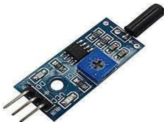
Figure 5 Vibration sensor
