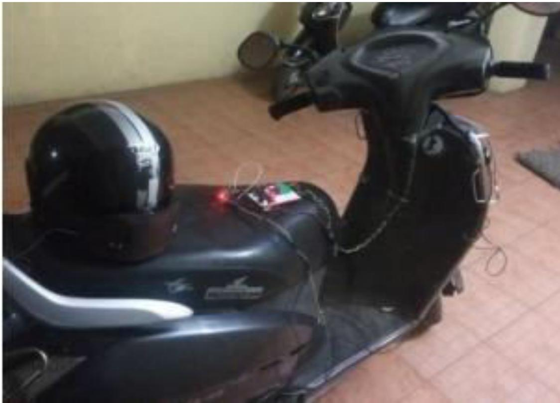
The best part about this project is that it doesn't work until it's worn since a limit switch has been added inside the helmet. Therefore it doesn't send messages if it's thrown or falls down. Also, it's calibrated such that it won't send messages for values due to speed breaker's or other small knocks.
