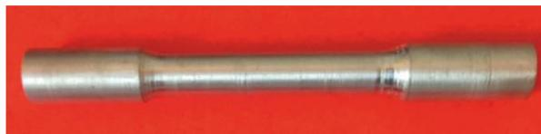
Figure shows Tensile testing sample
