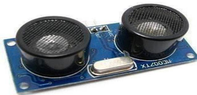
Fig 4.3 ultrasonic sensor
