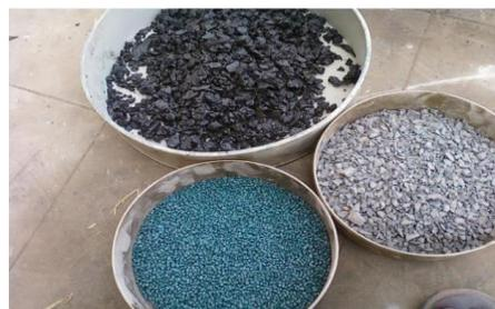
Figure 3: Aggregate, Shredded Plastic, & Plastic Coated Aggregate
