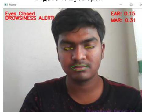
Figure 8. Eyes closed and drowsiness is triggered and alerted.
