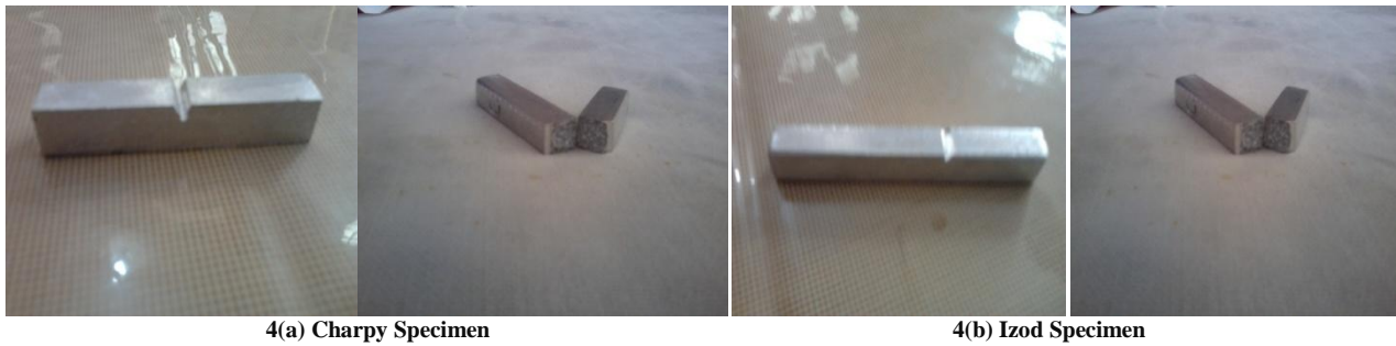
Figure 4: 4(a) Izod And 4(b) Charpy Test Specimen Before and After Testing
