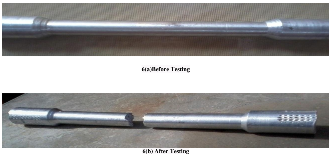
Figure 6: Tensile Test Specimen 6(a) Before and 6(b) After Testing
