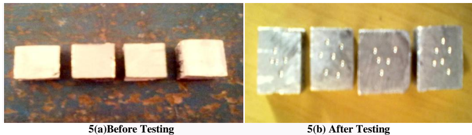
Figure 5: Hardness Test Specimen 5(a) Before and 5(b) After Testing
