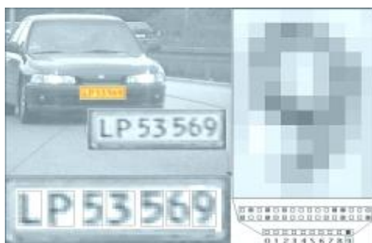
Fig.3.a. Locating the license plate on a digital image
