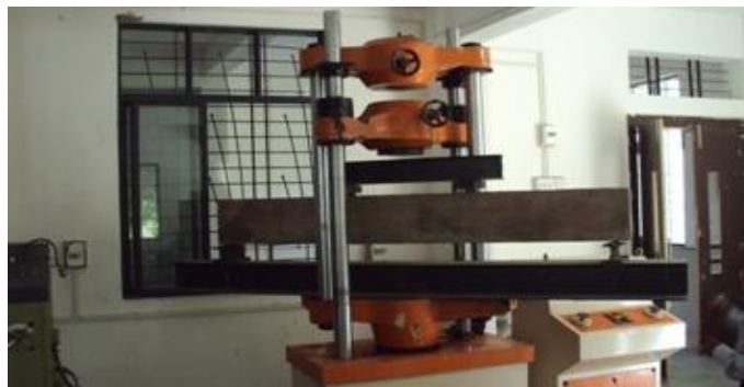
Fig.2 Test Setup for Beam Testing
