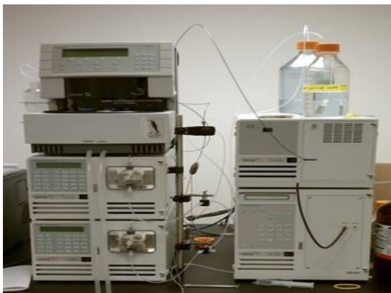
FIG 4:- H.P.L.C Instruments and components (Shimadzu-10x)
