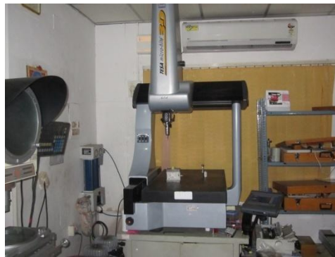
Fig. 7 Photograph of CMM used for measuring ovality of drilled holes
