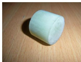
Fig. 1 Photograph of the GFRP rod manufactured by pultrusion process
