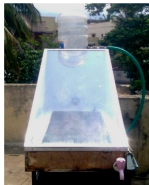
Fig. 1 Solar Still made up of GI Sheet
