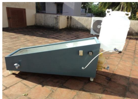
Fig. 2 Solar Still made up of Copper
