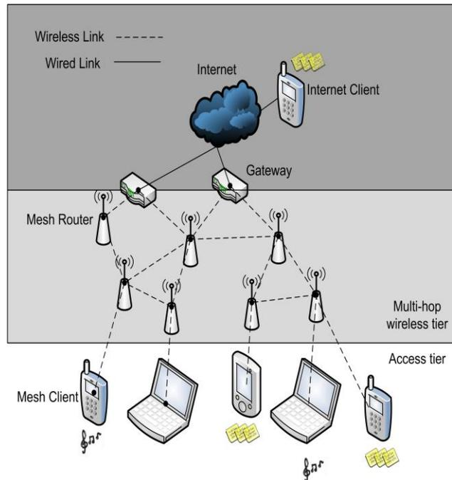
Fig. 1. Wireless Mesh Network Architecture
