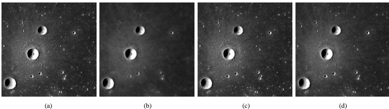
Fig.2 Image Smoothing (a) Input Image[11] (b) Image smoothing using morphology operation (size of structuring element is 2)(c) Image smoothing using Gaussian (d) Image smoothing using size of structuring element 1.
