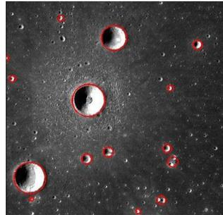
Fig.4 Detected Craters with Ellipse fitting
