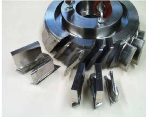
**Fig 5** Pre-machined BLISK demonstrator after extraction of blade blocks
