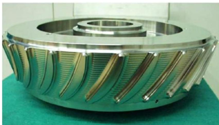
**Fig. 4** Disk for BLISK demonstrator
