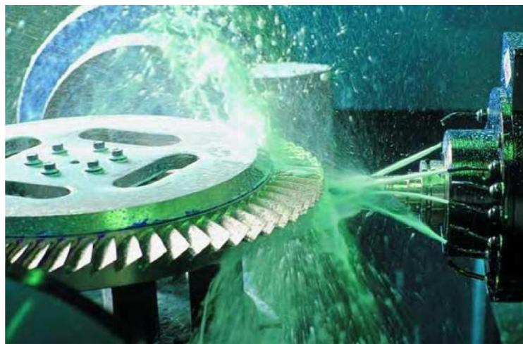
**Fig. 2.** BLISK machining by high-speed milling (courtesy of MTU Aero-Engines).
