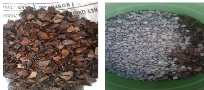
Fig.1 Sizes of coconut shell aggregate and normal aggregate
