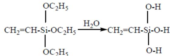
Fig. 2. Hydrolysis of silane. Reprinted with permission from Kalia, S. et al. [16]
