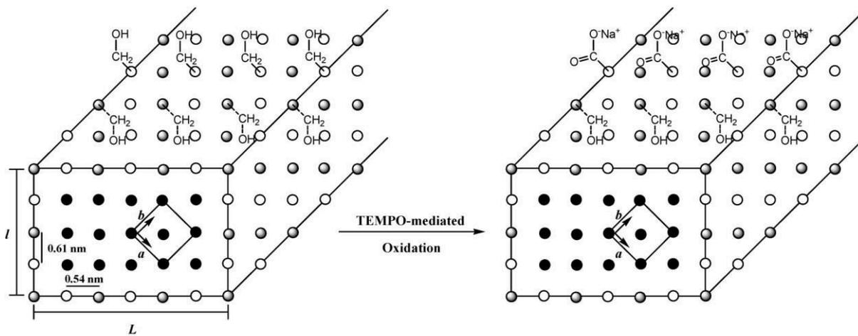
Fig 5. Scheme of TEMPO-mediated oxidation mechanism of the hydroxymethyl groups of cellulose (top, reaction scheme) and crosssectional representation of cellulose nanocrystal indicating the occurrence of the surface TEMPO-mediated oxidation of available hydroxyl groups (bottom, surface crystal representations). Reprinted with permission from the Reference [6]. Copyright 2010, American Chemical Society)
