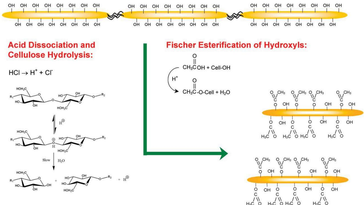
Fig. 1. Reaction scheme illustrating the one-pot (tandem) cellulose hydrolysis and esterification reactivity of hydroxyl groups. Reprinted with permission from Braun, B. et al. [7]. Copyright 2009 American Chemical Society.
