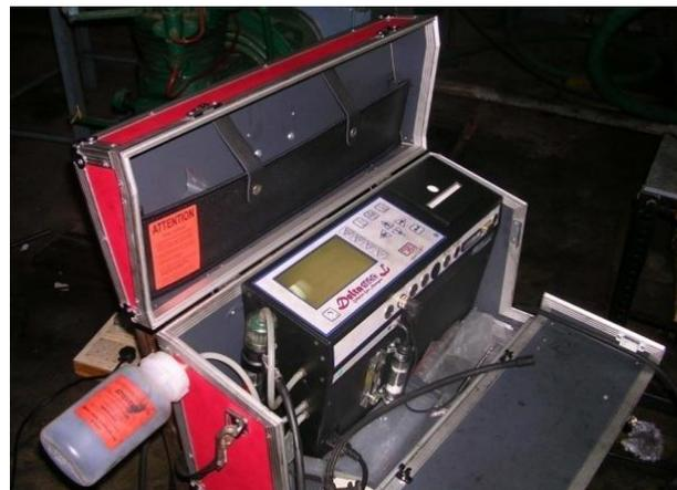
Figure 4: MRU Emission Monitoring System
