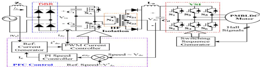
**Fig 2.1: Control Schematic Of Proposed Bridge-Buck PFC Converter Fed PMBLDCM Drive**
