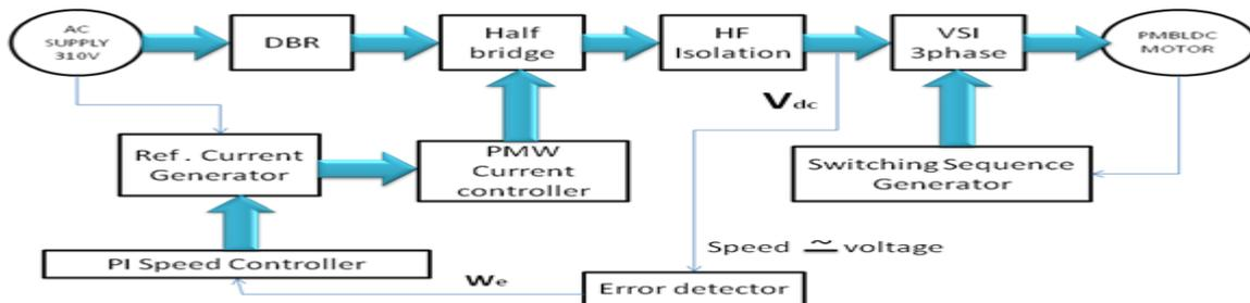
Fig 1.1: Block Diagram Of A Permanent Magnet Brushless Dc Motor Drive.
