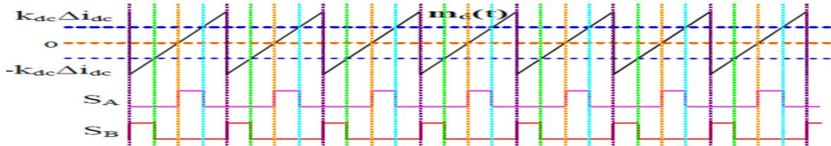
Fig 3.1: PWM Control Of The Buck Half-Bridge Converter
