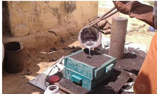
Fig: 5-Pouring of molten metal into the Mould
