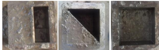
Fig 1 Step by step procedure of casting of vertical failure, diagonal failure and horizontal failure plane.
