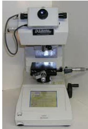
Fig.13 Vickers Microhardness Tester (Shimadzu)
