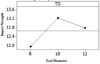
Fig. 7 Influence of Tool pin diameter on Impact Strength
