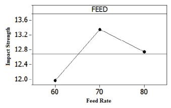
Fig.8 Influence of feed rate on Impact Strength
