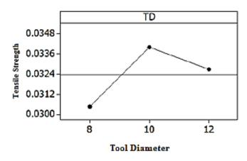
Fig. 4 Influence of Tool Pin Diameter on Tensile Strength
