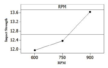
Fig. 6 Influence of RPM on Impact Strength
