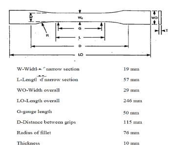
Fig. 1 ASTM Standard Tensile Test Specimen
