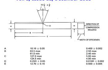
Fig. 2 ASTM Standard Impact Test Specimen
