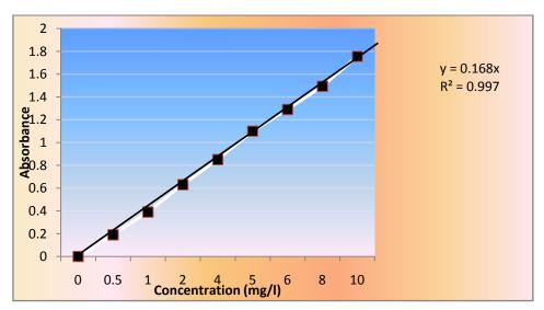
Fig. 4. Calibration plot for Methylene Blue at 660 nm
