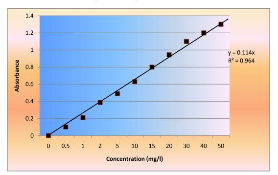
Fig. 5. Calibration plot for Congo Red at 500 nm
