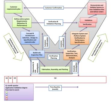
Fig. 9. V - model of system engineering processes for ICDI firm
