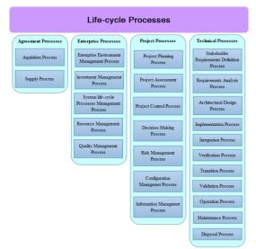
Fig. 1. Systems engineering life-cycle processes - ISO/IEC 15288
