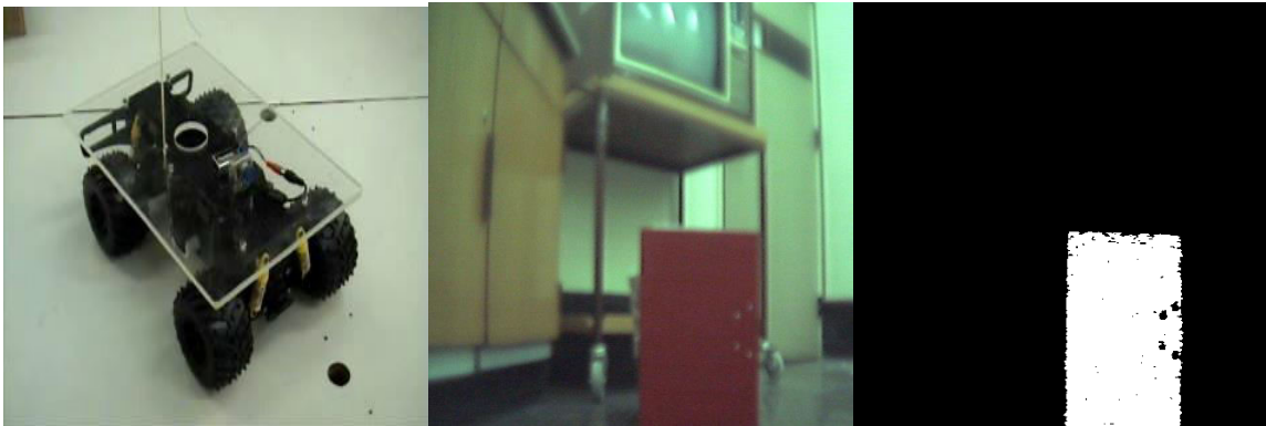
Fig.8 The robot image, (a) the images captured by the onboard camera, (b) and color-segmented image, (c) during one run of the vehicle.
