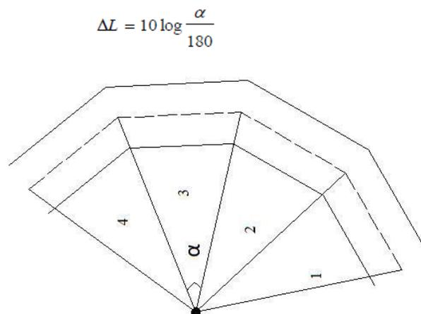
FIGURE 2. SCHEMATIC REPRESENTATION OF SEGMENTATION AT CURVES
