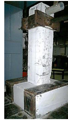
FIGURE 16. FAILURE PATTERN OF CDD6
