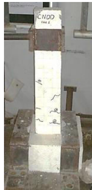
FIGURE 17. FAILURE PATTERN OF CNDD
