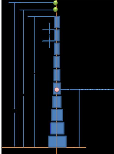
For a recommended pitch natural period shorter than 4 s, the 3P frequencies of wind turbine are overlapped and resonance might occur. To avoid this, the pitch natural period should be about 4 s [6]. The relationship between individual parameters and their effect on the natural period [4-7] are tabulated in Table 2, which can be used as an aid to control natural frequencies to the above stated limits.
