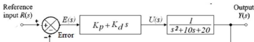
Figure (4) transfer function of velocity drive example
