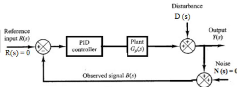
Figure (3) close loop system with no input R(s) and sensor noise
