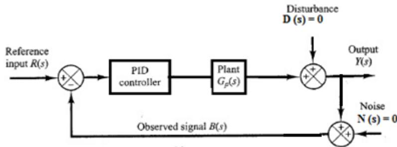
Figure (2) close loop system with no disturbance and sensor noise
