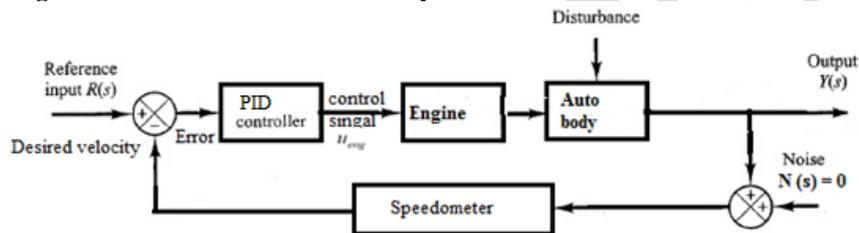
Figure (3) Vehicle drive through hills the aim is constant velocity
