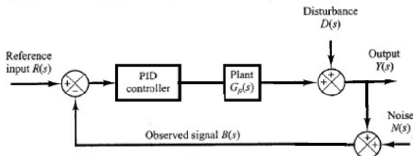
Fig. 1. Block Diagram of close loop system
