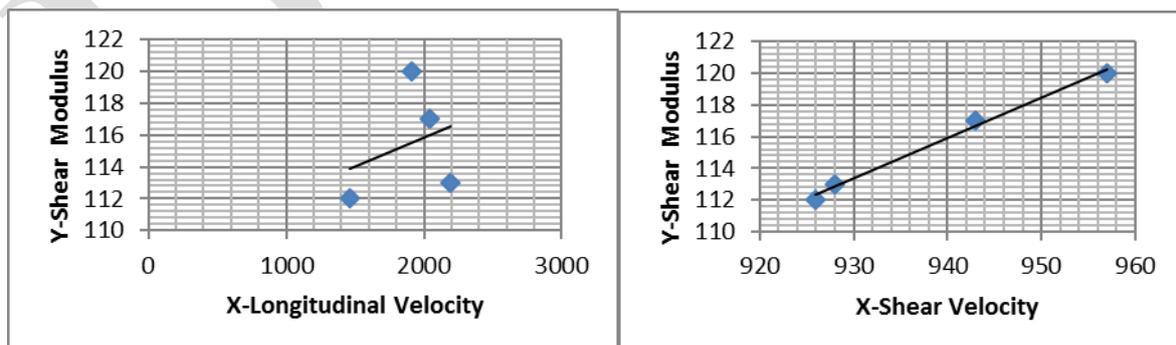
**Fig.10.**Correlation between Longitudinal velocity and Shear Modulus, correlation between Transverse velocity and Shear Modulus
