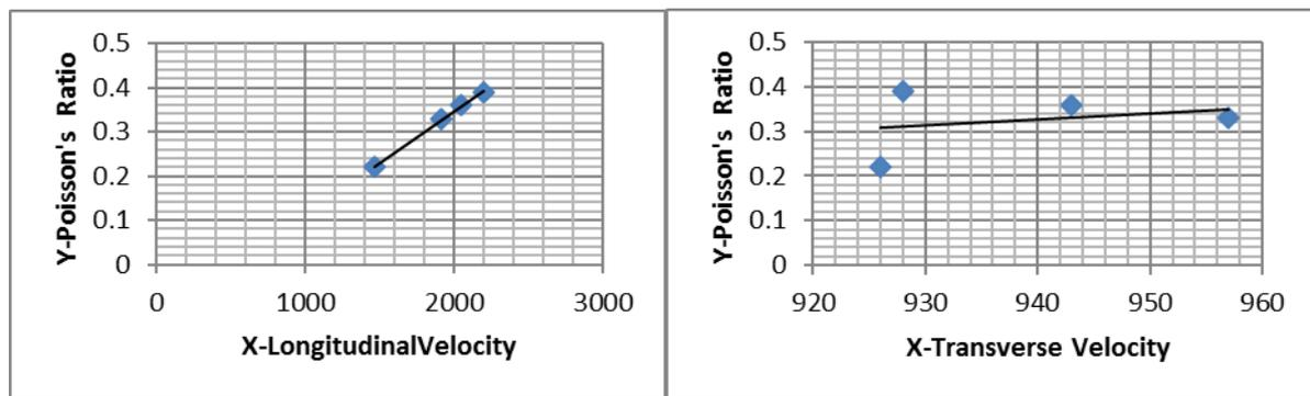
**Fig.11.**Correlation between Longitudinal velocity and Poisson’s Ratio, correlation between Transverse velocity and Poisson’s Ratio for the samples heated at different temperature.
