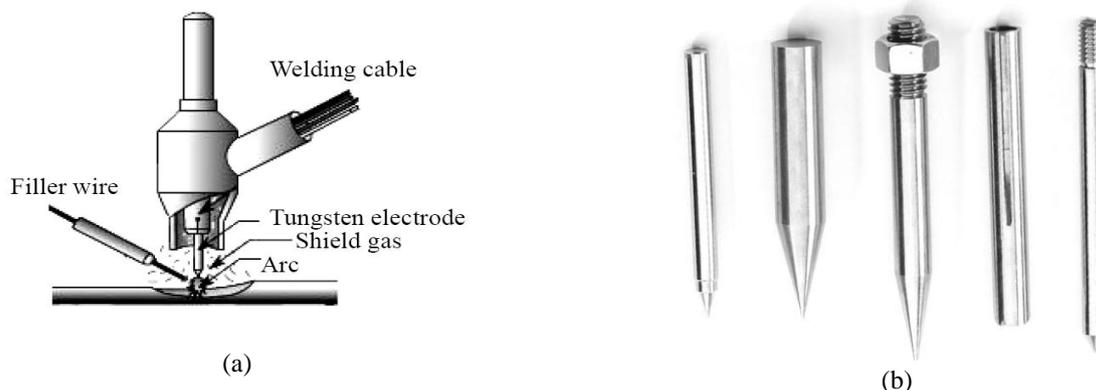
Fig. 1. (a) Schematic of TIG welding Process (b) Variety of tungsten electrodes
