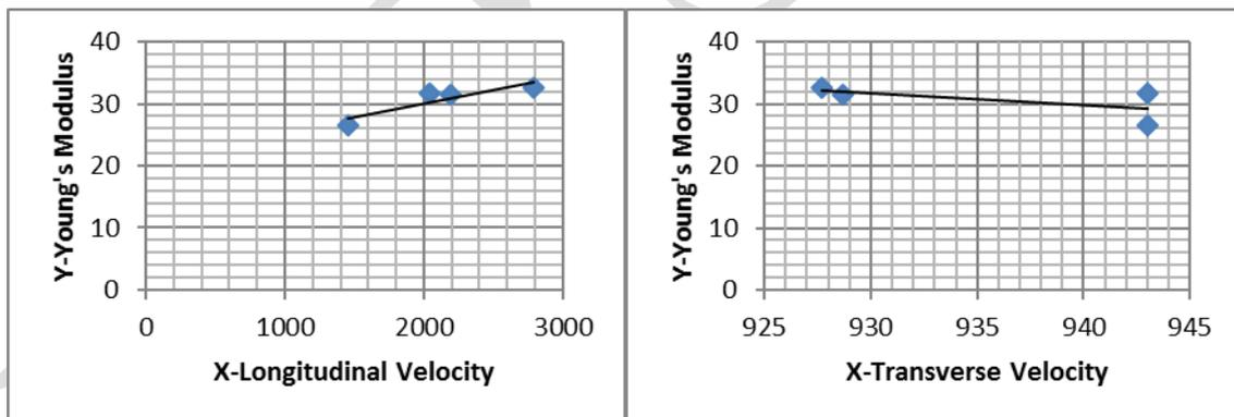
**Fig.4.**Correlation between Longitudinal velocity and Young’s Modulus, correlation between Transverse velocity and Young’s Modulus for the heat treated samples at 1500<sup>o</sup>C for different holding time.
