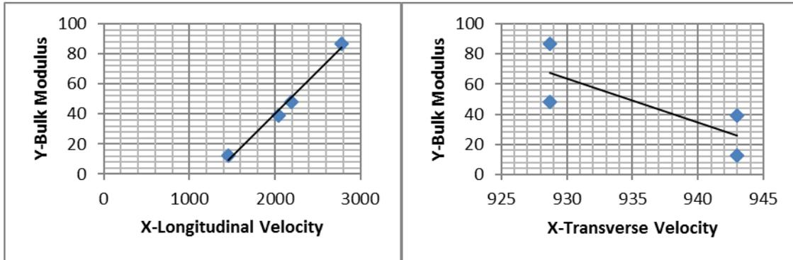
**Fig.5.**Correlation between Longitudinal velocity and Bulk Modulus, correlation between Transverse velocity and Bulk Modulus for the heat treated samples at 1500<sup>0</sup>C for different holding time.
