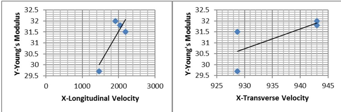
**Fig.8.**Correlation between Longitudinal velocity and Young’s Modulus, correlation between Transverse velocity and Young’s Modulus for the samples heated at different temperature.
