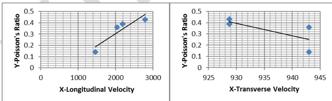
**Fig.7.**Correlation between Longitudinal velocity and Poisson’s Ratio, correlation between Transverse velocity and Poisson’s Ratio(1500 deg C)
