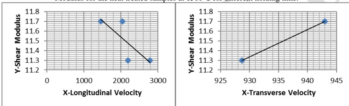
**Fig.6.**Correlation between Longitudinal velocity and Shear Modulus, correlation between Transverse velocity and Shear Modulus (1500 deg C)
