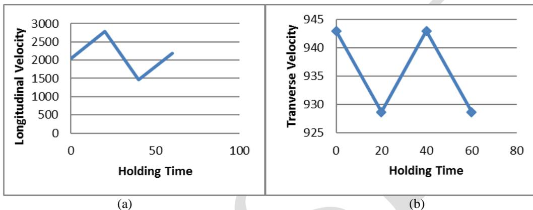
Fig.2. (a) Longitudinal velocity vs holding time at 1500 deg C (b) Transverse velocity vs holding time at 1500 deg C
