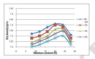
Figure 3: Variations in compaction curves.
