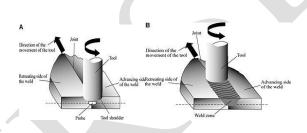
The welding of aluminium and its alloys has always represented a great challenge for researchers and technologists. Friction stir welding (FSW) is a new welding process that has produced low cost and high quality joints of aluminium alloys.
