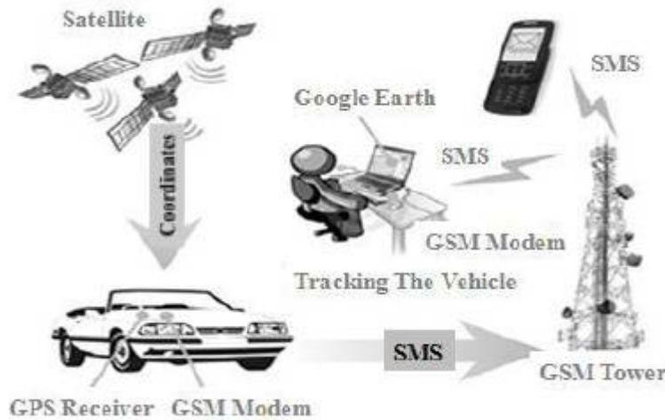
Fig.2. Block diagram of security system
