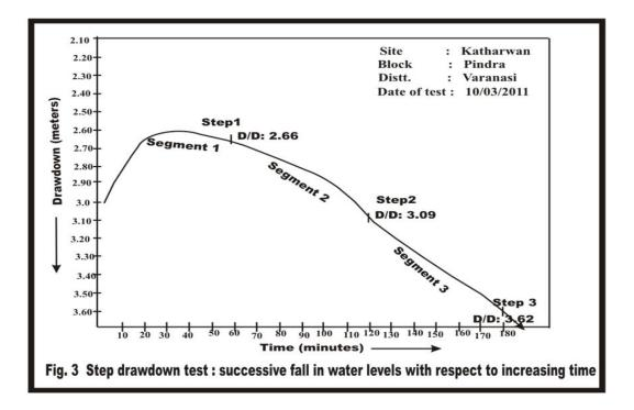
Fig.3: Step drawdown test showing the three step process. By increasing discharge rates for each step successively with respect to time; corresponding drawdown was measured which when plotted against increasing time, depicts the gradually falling water levels.
