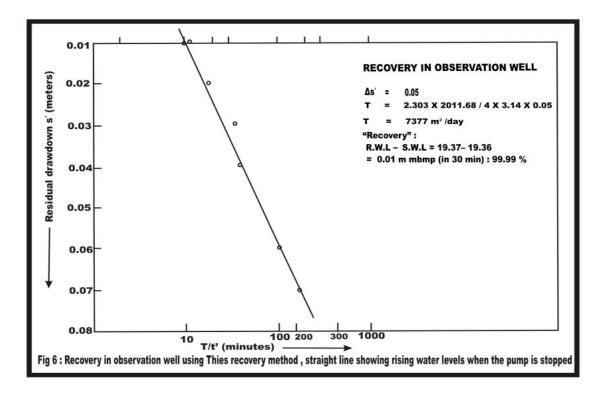
Fig.6: When the pumping had stopped; measurement are taken in an observation well to ensure the *Transmissivity* outcome which reveals in concept of suddenly rising water levels (termed as residual water levels), calculated using Thies' Recovery Method.
