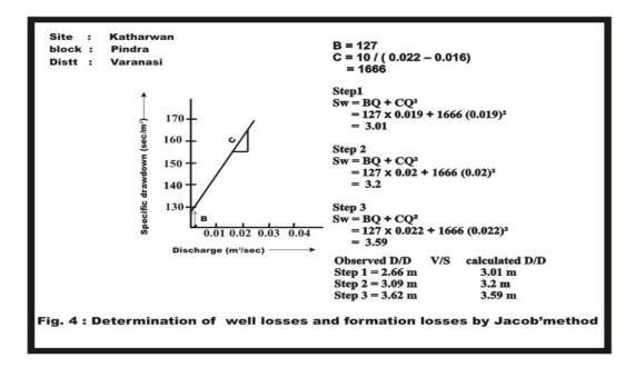
Fig.4: Determining the quantitative loss effect during step drawdown process by comparing actual observed drawdown (by tape measurements) with calculated drawdown using Jacob' method (described in text). It is essential in sense to convince with the accurate data analysis.
