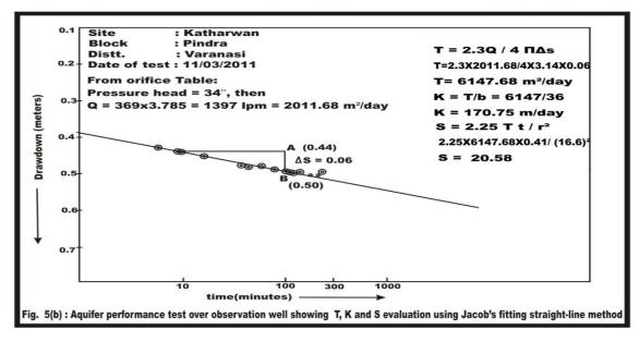
Fig.5: Showing result for an Aquifer performance test conducted over Pumping well or Exploratory well and Observation well respectively. Time vs. corresponding drawdown graph drawn using Cooper-Jacob straight line method to calculate hydraulic parameters: Transmissivity, hydraulic conductivity and Storativity.
