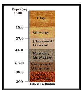
Fig. 2: Subsurface lithology through an exploratory well showing litho unit with their corresponding thickness.
