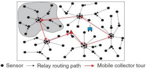
Sensor → Relay routing path → Mobile collector tour
