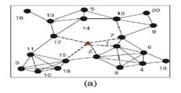
Figure 5 An example to illustrate the PB-PSA algorithm (N=20, d=2) Network Configuration
