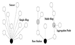
Figure 2 Single-Hop and Multi-Hop transmission
