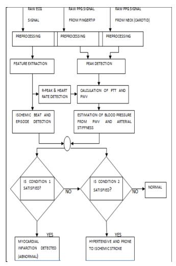
Fig.8 Execution Flow of the Proposed System
