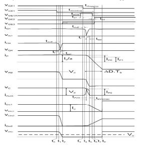
Fig. 2. Key waveforms concerning the operation stages in the proposed PSFB PWM converter.
