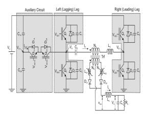
Fig. 1. Proposed PSFB PWM converter.
