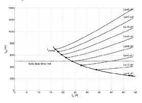
Fig. 4. Characteristics of the proposed converter for CP = 25 nF.
