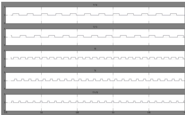
Fig. 7 switching pattern of Single Phase Seven Level Inverter
